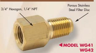
Brass with 1/8" thick micro-metallic stainless steel filter (max pressure 1500 PSI) Available 1/4" NPT only. Specify **WG41** for air. Specify **WG42** for water or light oil. **WS41/WS42** Stainless steel body instead of brass.
