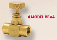
Brass, 1/4" NPT female connections only. Suitable for 600 PSI at 300° F maximum; for water, oil or gas service. **SSV4** 316SS body rated to 5,000 PSI.
