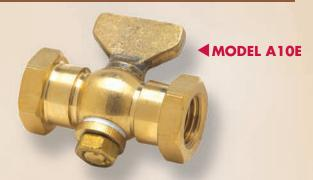
In polished brass for pressures to 200 PSI hydraulic, 1/4" NPT female connections with hex shoulders.
