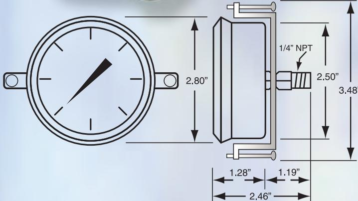
The Glycerin filling in liquid filled gauges helps dampen the effects of pulsation and vibration. While also perpetually lubricating the movement and keeping contaminants away, the liquid extends the life of the gauge.
